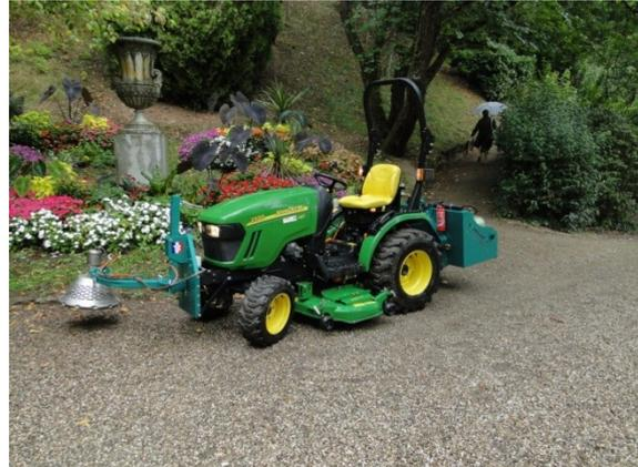
The **bell**, mounted on an extendable arm, **moves around and retracts** when it comes into contact with an obstacle (e.g. a traffic sign). The inward and rearward clearance is approximately 300 mm
