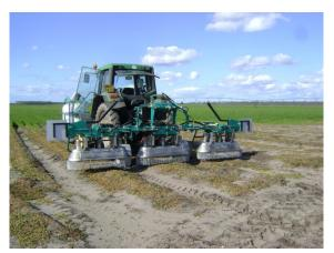
opening and closing of the side arms). The management of the height and level of the diffusers in relation to the ground is carried out via ultrasonic sensors controlling the electrodistributors automatically.
